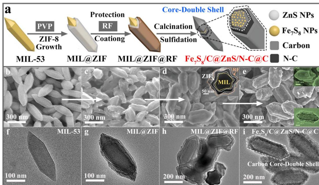
Fig. 8 (a) Synthesis of 3D core-shell  $\text{Fe}_7\text{S}_8/\text{C}@\text{ZnS}/\text{N}-\text{C}@\text{C}$ ; SEM/TEM images of (b) and (f) MIL-53, (c) and (g) MIL@ZIF, (d) and (h) MIL@ZIF@RF and (e) and (i)  $\text{Fe}_7\text{S}_8/\text{C}@\text{ZnS}/\text{N}-\text{C}@\text{C}$  ((a)–(i)) reproduced with permission from ref. 145, copyright© 2020, WILEY-VCH Verlag GmbH & Co. KGaA, Weinheim).
